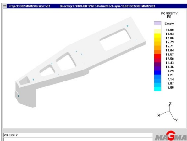
Fig. 2 The distribution of porosity above 5% for compositions S1 and S3 given in Table 1
