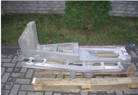
Fig. 4. Casting of the base weighing 102 kg. GJS 400-15
